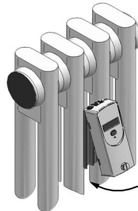
Push the seal pre-installed by Sontex in the slot of the housing, then press until the seal clicks into the aluminium back plate.
