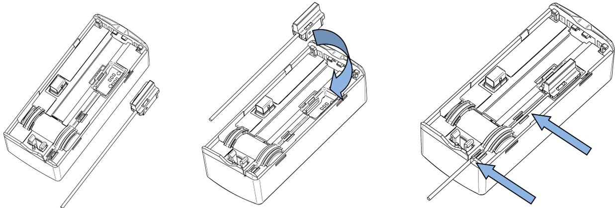
Return the heat cost allocator and plug the connector of the remote sensor into the interface inside the heat cost allocator.
