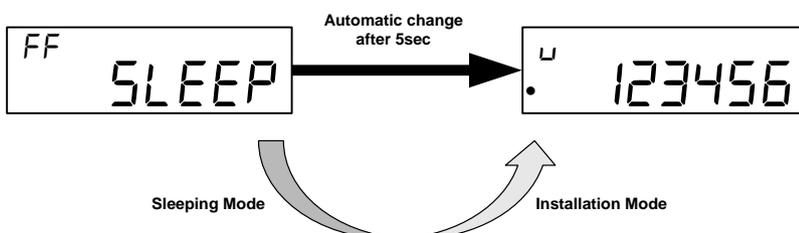
The **•** symbol indicates that the heat cost allocator is in installation mode.
