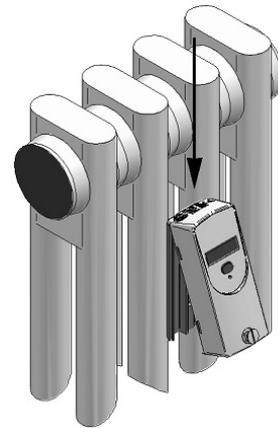
The heat cost allocator is placed on the aluminium back plate in the direction of the arrow.
