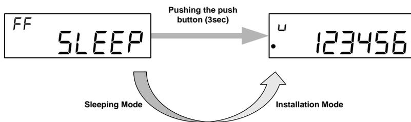
The • symbol indicates that the heat cost allocator is in installation mode.
